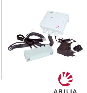
GEWA Andromeda BED is an IR receiver with which it is possible to control the functions of a motorized bed wirelessly via a GEWA IR transmitter. The receiver has 8 relay outputs, that can control a maximum of 8 functions of a bed: the head end, the foot end, knee part and the whole bed up/down.
